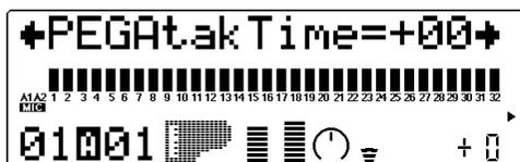
This determines the Attack Time of the Pitch EG, or how long it takes for the pitch to return to normal (from the pitch value set in Initial Level above).
