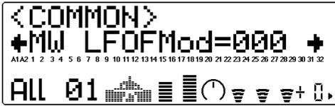
This determines how widely the Filter (page 135) is modulated by the LFO (low frequency oscillator). This is generally controlled from a modulation wheel on a MIDI keyboard, and depending on the Voice used, it creates a “swoosh” or “wah-wah” filter sweep effect. Higher values result in deeper filter modulation, creating a more pronounced filter sweep effect.
