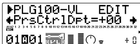
Sets the amount of variation produced by the controller assigned to pressure. The higher the value the greater the variation. Positive values cause an increase in pressure in response to higher controller values (e.g., increased breath pressure or higher modulation wheel position), while negative values cause a decrease in pressure in response to higher controller values.
