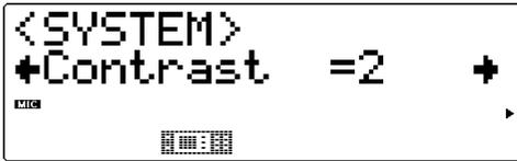
This determines the contrast of the display. Adjust this as necessary for optimum visibility. (At extreme settings, the display may not be readable.)
