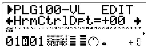
Sets the amount of variation produced by the controller assigned to the harmonic enhancer. The higher the value, the greater the variation. Positive values cause an increase in harmonic enhancer depth in response to higher controller values (e.g., increased breath pressure or higher modulation wheel position), while negative values cause a decrease in harmonic enhancer depth in response to higher controller values.
