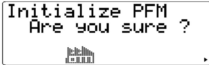
One of the four parameters above will be available, depending on the currently selected Sound Module mode: XG, TG300B, C/M or PFM. Initializing this parameter restores the original settings for the selected mode.
