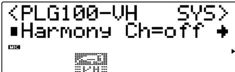
This determines the MIDI channel over which the Harmony effect is controlled. For example, when this is set to the same value as the MIDI transmit channel of a connected MIDI keyboard and the Vocoder or Chordal Harmony Type is selected (page 147), you can use the keyboard to “play” harmonies. (See page 77.)
