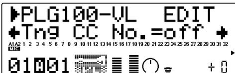
“Tonguing” simulates the half-tonguing technique used by saxophone players by changing the “slit” of the reed. The slit is the space between the tip of the reed and the mouthpiece. The “Tng CC No.” parameter specifies the controller to be used for tonguing control. When set to “off” no tonguing is applied.
