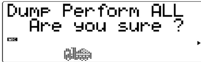
This transmits the selected MU100R Performance data to the connected device. (Use the VALUE  $\ominus/\oplus$  buttons or data dial to select the type/amount of data to be transmitted.)
