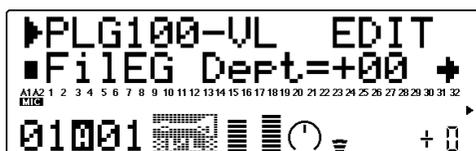
Sets the amount of variation produced by the controller assigned to dynamic filter. The higher the value the greater the variation. Positive values cause an increase in filter cutoff frequency in response to higher controller values (e.g., increased breath pressure or higher modulation wheel position), while negative values cause a decrease in filter cutoff frequency in response to higher controller values.
