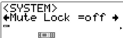
This determines whether or not the Part Mute status of the MU100R is reset when receiving a **GM System On** or **XG System On** message. Generally, this message is automatically transmitted to the MU100R as part of General MIDI song data. When Mute Lock is set to **off**, this resets the Mute status of the Parts on the MU100R. If you want to keep the current Mute settings and disable this reset, set Mute Lock to **on**. (For more information on the Mute function, see page 85.)
