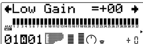
This determines the level of the selected frequency (in Low Freq above). Positive values boost the level of the selected frequency and negative values attenuate it.
