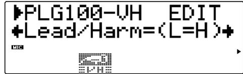
This determines the relative balance of the lead and harmony voices. For most pop song applications, this should be set to “L=H” or a slightly higher lead level (such as “L10>H” or more).
