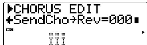
This determines the level of the Chorus signal sent to and processed by the Reverb effect. A setting of 000 results in none of the Chorus-processed signal going to the Reverb.
