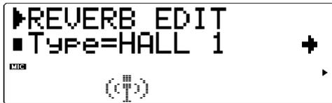
This determines the Reverb Type. Each Reverb Type has different values for the rest of the Reverb parameters; for example, Basement has a Reverb Time of 0.6 seconds, while Canyon has a Reverb Time of 12.0 seconds.
