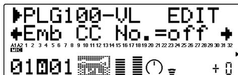
“Embouchure” corresponds to the tightness of the lips against the reed or against each other. In a string instrument Voice, embouchure corresponds to how strongly the bow is pressed against the string. This affects both pitch and timbre. The “Emb CC No.” parameter specifies the controller to be used for embouchure control. When set to “off,” medium embouchure is applied at all times.
