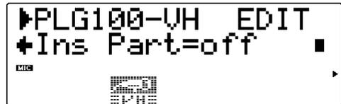
This determines the Part to which the Harmony effect is applied. For example, to apply Harmony to a microphone input through A/D INPUT 1, set this to “AD01.” When set to “off,” the Harmony effect is cancelled.
