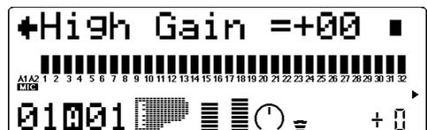
This determines the level of the selected frequency (in High Freq above). Positive values boost the level of the selected frequency and negative values attenuate it.
