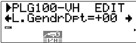
This determines the quality or character of the lead voice, and depends on the setting made in Lead Gender Type above. (This parameter has no effect when Lead Gender Type is set to “off.”) Extreme negative or positive values result in pronounced distortion of the voice quality. Also, the effect may vary according to the quality, character and pitch of the actual voice. Experiment with this to find values that sound most natural (or unnatural, if you prefer).
