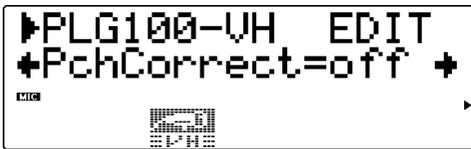
This determines whether the pitch of the lead voice is controlled by MIDI note data or not. When this parameter and Lead Gender are set to “on,” the pitch of the lead voice is “corrected” to the pitch of the received MIDI note on Melody Channel (page 171).
