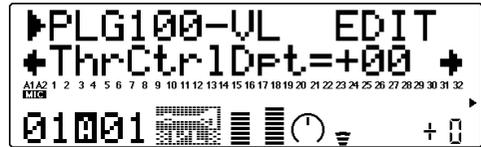
Sets the amount of variation produced by the controller assigned to throat formant. The higher the value, the greater the variation. Positive values cause an increase in throat formant effect in response to higher controller values (e.g., increased breath pressure or higher modulation wheel position), while negative values cause a decrease in throat formant effect in response to higher controller values.
