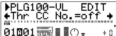
“Throat Formant” controls the characteristics of the simulated player’s lungs, trachea, and oral cavity and can add a realistic “roughness” to the sound. The “Thr CC No.” parameter specifies the controller to be used for throat formant control. When set to “off”, no throat formant variation can be produced via a controller, but a continuous throat formant value is determined by the “ThrCtrlDpt” parameter, below (negative values increase the throat formant level).
