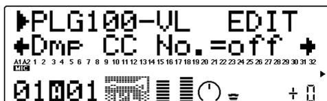
“Damping” simulates the effect of damping due to losses within the body of a wind instrument or in a string due to air friction. This affects both pitch and timbre. The “Dmp CC No.” parameter specifies the controller to be used for damping control. When set to “off,” no damping variation can be applied via a controller.
