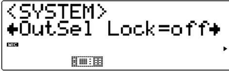
This determines whether or not the Output Select settings (pages 113, 118) are reset when receiving a **GM System On** or **XG System On** message. It also determines whether the Output Select setting for a Part can be edited via MIDI or not. If you want to “lock” the Output Select settings and keep them from being changed, set this to “on.”
