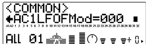
This determines the degree to which Assignable Controller 1 (AC1) affects the LFO modulation of the Filter. This creates a regular and continuous “wah-wah” or filter sweep effect. The higher the value, the greater the LFO filter modulation. (The control number used for AC1 is set in the Assignable Controller 1 Control Change Number parameter above.)
