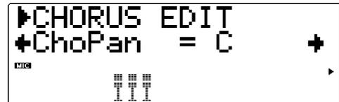
This determines the Pan position of the Chorus sound, or where it appears in the stereo image.
