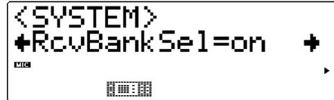
This determines whether Bank Select messages are received or not. Bank Select messages can be sent from another MIDI device to change the banks of Voices on the MU100R. (See page 31.) The On setting allows Bank Select messages to be received.
