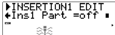
This determines the Part to which the Insertion effect is applied. Insertion can be applied to only one Part at a time.
