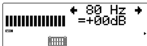
The remaining EQ parameters let you set the level of each of the five frequency ranges: low, low-mid, mid, high-mid and high. The bars in the display show the EQ settings as a frequency “curve,” with peaks indicating level boosts in the frequency range and valleys indicating level cuts. A setting of 00 dB corresponds to no level change.
