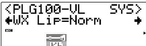
WX-series Wind MIDI Controllers produce pitch bend data ranging from “-16” to “+32” in response to lip (reed) pressure. The WX Lip parameter determines whether these values are used as is (“Norm”), or expanded to a full “-64” through “+63” range (“Expd”). This is also effective for pitch bend data transmitted from devices other than those of the WX-series.
