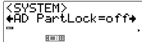
This determines whether or not the current parameter values and Variation effect settings of the A/D Parts are reset when receiving a **GM System On** or **XG System On** message. If you want to keep the current parameter values and Variation settings of the A/D Parts, set Mute Lock to **on**. (This parameter has no effect in the Performance mode.)
