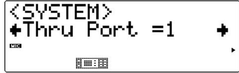
Some MIDI devices and sequencers are capable of transmitting data over several MIDI “ports,” effectively breaking the 16-channel barrier. When this data is received via the TO HOST terminal on the MU100R, this parameter determines which MIDI port’s data will be routed through the MIDI OUT terminal. This allows you to connect another multi-timbral tone generator to the MU100R and play back data over 48 independent MIDI channels — 32 on the MU100R and another 16 on the connected tone generator.
