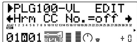
The Harmonic Enhancer can vary the harmonic structure of the sound over a wide range. The “Hrm CC No.” parameter specifies the controller to be used for harmonic enhancer depth (wet/dry balance) control. When set to “off”, no harmonic enhancer depth variation can be applied via a controller.
