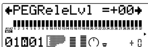
This determines the final pitch of the Part's Voice, or the pitch that is reached after the note is released. A setting of 00 corresponds to normal pitch.
