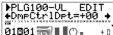
Sets the amount of variation produced by the controller assigned to damping. The higher the value, the greater the variation. Positive values cause a decrease in damping in response to higher controller values (e.g., increased breath pressure or higher modulation wheel position), while negative values cause an increase in damping in response to higher controller values.
