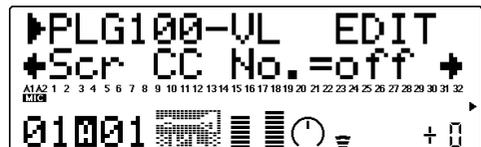
“Scream” drives the entire system into chaotic oscillation, creating effects that can only be achieved with physical modeling technology. The “Scr CC No.” parameter specifies the controller to be used for scream control. When set to “off”, no scream variation can be produced via a controller, but a continuous scream value is determined by the “ScrCtrlDpt” parameter below. (Negative values increase the scream level.)
