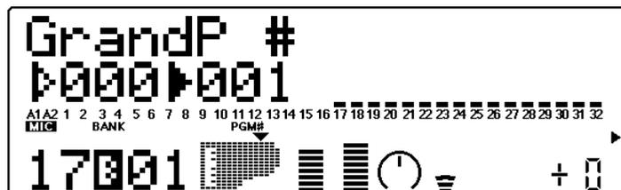
For this example, select Part 1. Press the appropriate button until “01” appears in the PART section of the display.
