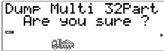
This transmits the selected MU100R Multi Part data (including System, Effect and EQ data) to the connected device. (Use the VALUE  $\ominus/\oplus$  buttons to select the type/amount of data to be transmitted.)
