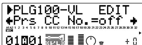
“Pressure” corresponds to the amount of breath pressure applied to a reed or mouthpiece, or the speed of the bow applied to a string. Pressure variations affect both volume and timbre. The “Prs CC No.” parameter specifies the controller to be used for pressure control. When set to “off” maximum pressure is applied at all times.
