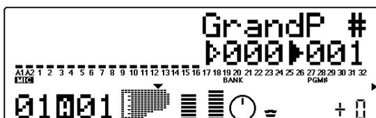
This shows the level meters at their maximum height, but only displays half of the Parts.
