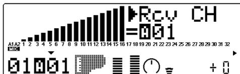
This determines the MIDI IN port (A or B) and the receive channel (1 — 16) for the selected Part.
