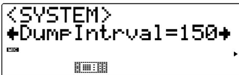
This determines the length of time the MU100R pauses when sending blocks of data in the Dump Out functions. If the receiving device fails to process the data or displays a “buffer full” type message, try setting this parameter to a higher value and send the data again.
