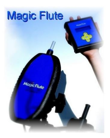
The Magic Flute is not only an instrument but also acts as the remote control for the Control Module (sip & puff).
